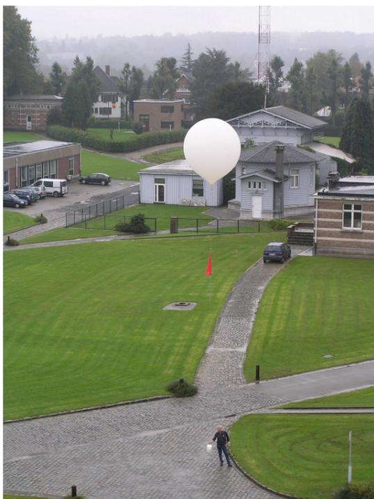
Figure 2: The launch of an ozone sounding by a radiosonde attached to a weather balloon, here at Uccle.
