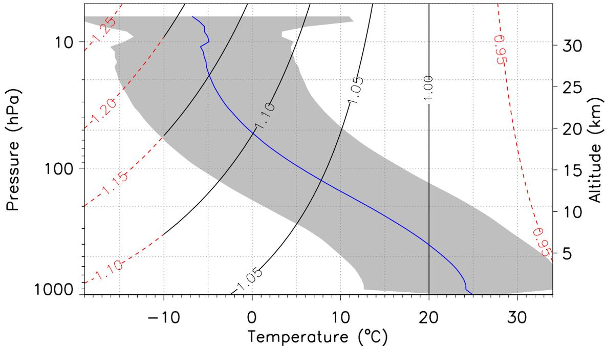
Figure 4: Mean ratios between the time needed to pump 100 ml at temperature  $t$  and pressure  $p$  and the time at 20°C with BM pumps. The solid black lines result from interpolation between the measured points with a polynomial (Eq. (15)); the dashed red lines indicate extrapolation. The blue line and shaded area show the mean and  $2\sigma$  of the box temperatures for BM observed between 1990 and 1998.
