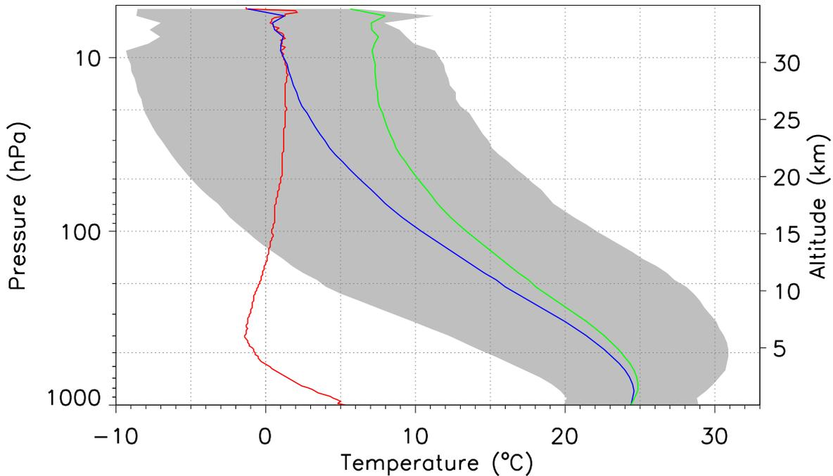
Figure 2: Mean box temperature during ascent (blue line) and descent (red line) from the BM soundings during 1990 and 1991. The grey zone indicates the  $2\sigma$  limits corresponding with the variations of the box temperature during ascent. The green line represents the adjusted mean box temperature applied before 28 April 1989
