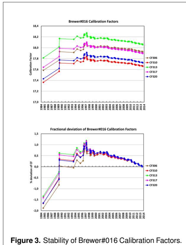
Figure 3. Stability of Brewer#016 Calibration Factors.
