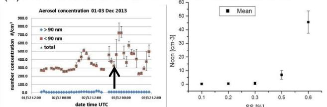
**CPC number concentrations** were 385 ± 72 cm<sup>-3</sup> during summers and 91 ± 64 cm<sup>-3</sup> for autumn 2013. The **Count Median Diameters** from the **LAS** measurements were in the range 110 – 140 nm and the presence of particles above 2 μm was negligible.
